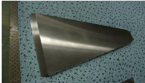
Figure 2.7. Example of a tungsten plate used for the assembly of prototype IV.
