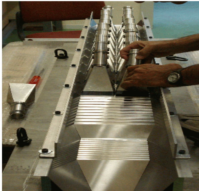
Figure 2.6. Assembly of light guides onto W/Q sampling units of prototype IV.
