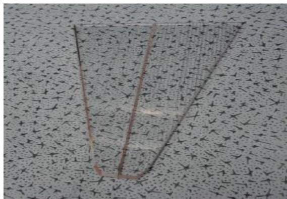
Figure 2.8. Example of a quartz plate used for the assembly of prototype IV.
