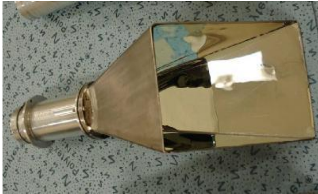
Figure 2.9. Air-core light guide designed for prototype IV and reflecting foil covering inside.
