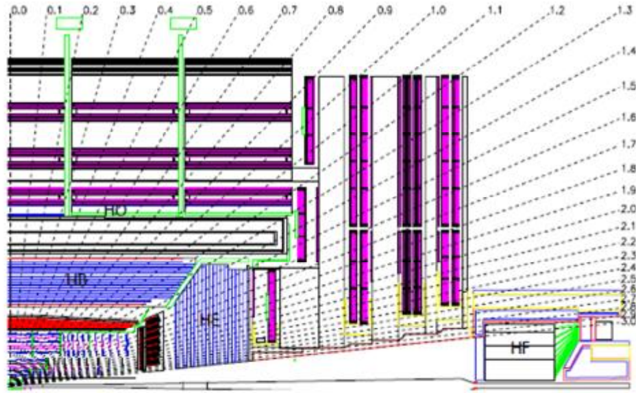
Figure 2.14. Longitudinal view of HCAL indicating the locations of the HB, HE, HO and HF calorimeters (CMS Collaboration, 2008, JINST 3 S08004).
